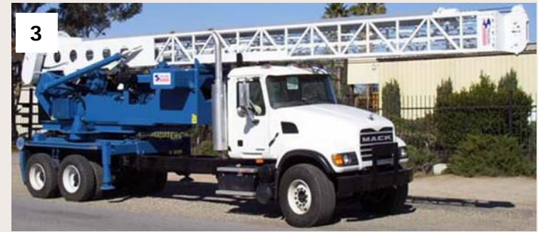
Conductor rig mobilizes to pad
